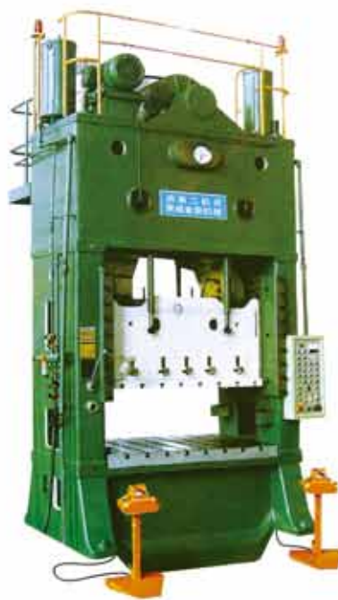
JD36-160型闭式双点单动压力机 JD36-160 Straight side double point single action press
