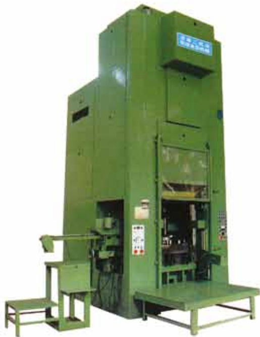
J89-400型立式肘杆冷挤压机 J89-400 Type vertical knuckle joint cold extrusion press
